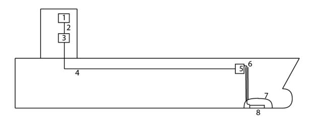
The sensor cable pipe (orifice tube) on the housing is part of the ship hull and has to reach above waterline (CWL=Construction water line.)
